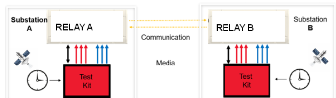
Fig. 1. Simultaneous secondary injection started by a trigger signal generated by two GNSS equipment in the two substations.
